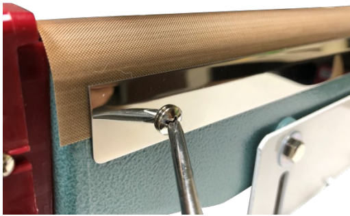
Figure 7. Loosen screws on PTFE plate.
