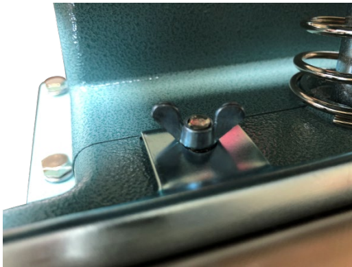
Figure 10. Loosen knob to remove the PTFE roller.
